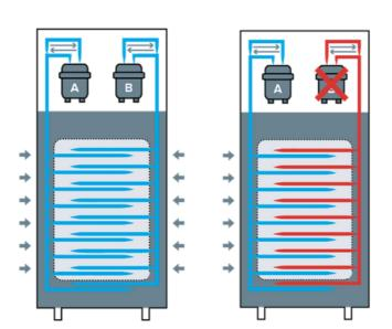
In case of a failure, the TRUE DUALTM technology maintains a stable temperature of +4 °C and protects the blood.
