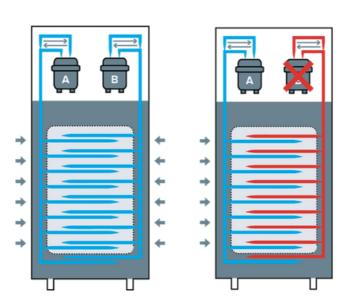
In case of a failure, the TRUE DUALTM technology maintains a stable temperature of +4 °C and protects the blood.
